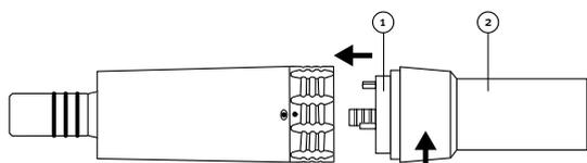
Use MK-dent Premium Service Oil to lubricate the o-rings on the tubing.
