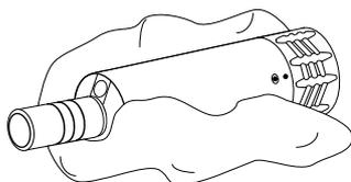
Spray disinfecting solution on a cloth and swipe off the motor. See manufacturers' manual for contact time. Only use DGHM/VAH listed chemical disinfectants for spray and wipe disinfection.
