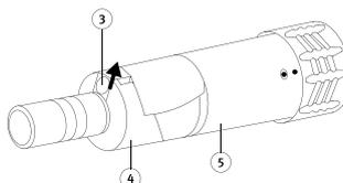
Press the porter 4 to the body 5 and push the LED 3 with screw driver in direction of arrow out of the socket. Take it out.
