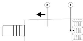
Push button 1 and pull off sleeve 2 from socket and take it out.
