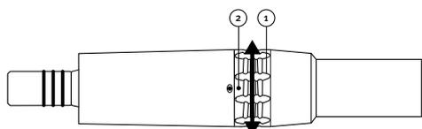
Turn the regulating sleeve 1 right or left to regulate the spray water.
