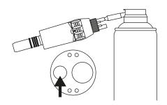
Use "MK-dent Premium Service Oil" for care and lubrication. Remove the Air Motor from the tubing, attach the enclosed MK-dent oil adapter on the oil can and spray for 1-2 seconds in the smaller one of the two large pipelines (see drawing).
