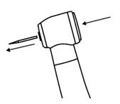
→ Use your thumb to press the button firmly after the rotating instrument has come to a complete stop and pull it out at the same time.
