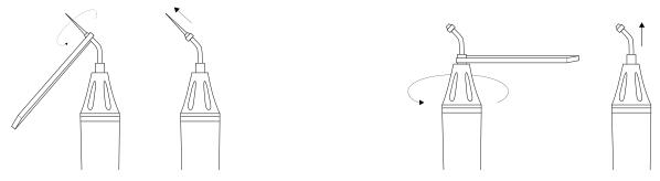
To remove the file, place the MK-dent Endo Torque onto the file holder and turn anticlockwise to loosen the connection.
