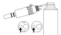
Use "MK-dent Premium Service Oil" for care and lubrication. Remove the Air Motor from the tubing, attach the enclosed MK-dent oil adapter on the oil can and spray for 1-2 seconds in the smaller one of the two large pipelines (see drawing).
